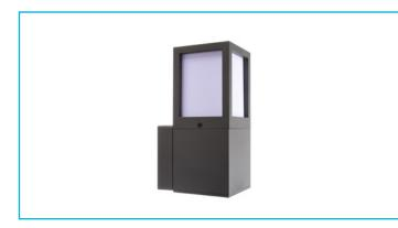
The FACADO wall light is our flexible solution for outdoor lighting. Two cable entry points allow for easy feed-through wiring. The removable mounting plate with plug connector and the screwless connecting terminals allow for quick and easy installation. The newly designed lamp head provides significantly improved illumination. IP65 degree of protection ensures impressive weather resistance.
